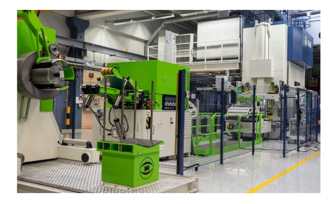
Compared to a traditional eccentric press, the structure of a servo press is different: for example, the motor, the clutch and the flywheel have been replaced with a servo motor. The operating system of a servo press is very versatile, as it has to control even the smallest movements of the servo motors. These are some of the great advantages servo presses, compared to an eccentric press.
